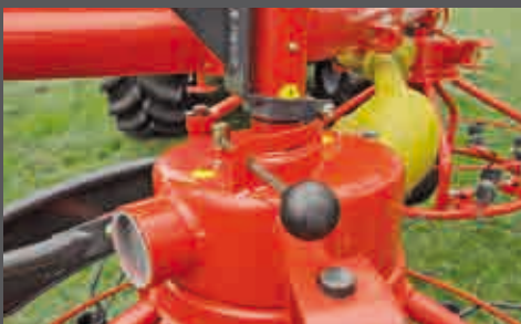
Lever for reversing rotor rotation and instruction decal (Haybob 360)
