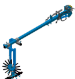
Finger hoe Hydraulic lift
