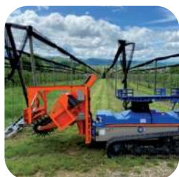
The Needle Harrow soil loosening system
