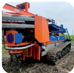
The Power Harrow ground cultivating system
