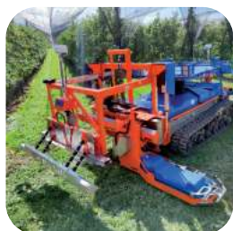
The Side Lawn Mower for mulching branches and cutting grass between and around the roots
