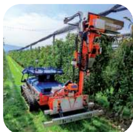
The Horizontal and Vertical Cutter for pruning branches vertically and horizontally
