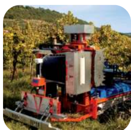
The Leaf Remover leaf removal system
