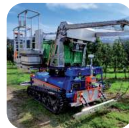
The Harvesting System adjustable moving shelves, frontal uploader and basket downloader
