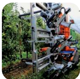
The Apple Picker harvesting system for fruits which imitates the movements of human hands
