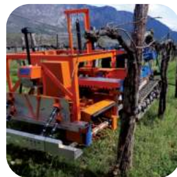
The Side-Trimmer weeding system for cleaning around the trunks
